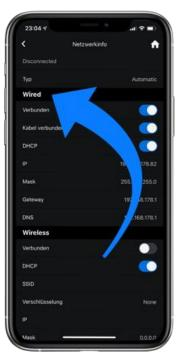
**NOTE**: If you don't see an available device, check that the network cable is installed correctly and that the AVM device is on the same network/Wi-Fi network as your smartphone or tablet. Next, drag the view down a bit in the **RC X app** to search for available devices again. Please also note that the **RC X app** is only compatible with AVM models with integrated AVM X-STREAM engine®. An up-to-date model overview can be found at: www.avm.audio/rc-x-app.
