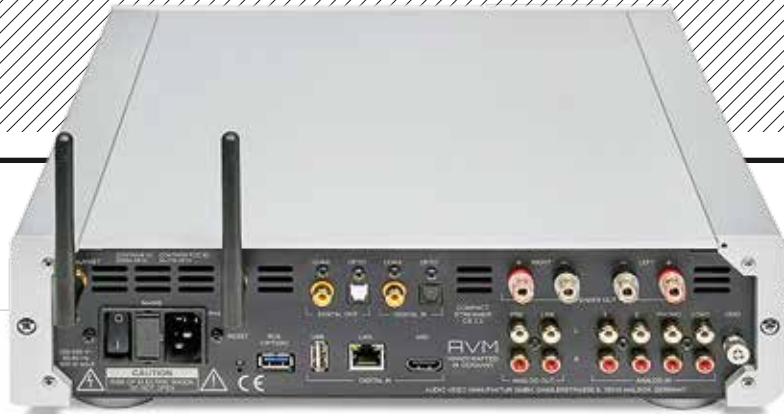
ABOVE: Two analogue line ins are joined by MM/MC phono (custom loading via adjacent RCAs) and digital in on wired/wireless LAN, BT, HDMI (ARC) and USB-A (for HDD connection). Digital in/out is available via coax/optical alongside fixed/variable preamp outs (RCAs) and a pair of 4mm speaker cable binding posts
